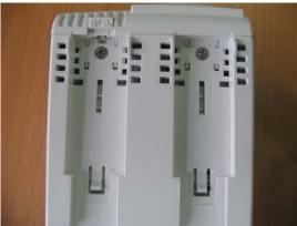
2. Take off the front cover of the CO<sub>2</sub> module by referring to the procedure as described in *5.6.1 Disassembling the ICG Module*. Then press the two clips about 1mm and take off the housing.
