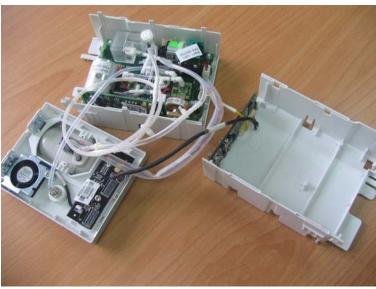
4. Take out the infrared communication board and disconnect all the cables from it.
