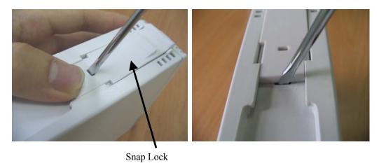
3. Unscrew the M3×6 screw. Then press down, in turn, the two clips that engage the front cover. At the same time, pull off the front cover carefully to avoid damaging the cables.
