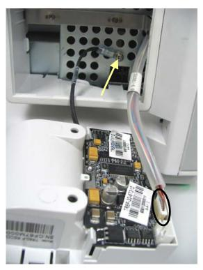
4. Unclench the two clips and meanwhile take out the recorder drive board. Pay attention to the snap in the front.
