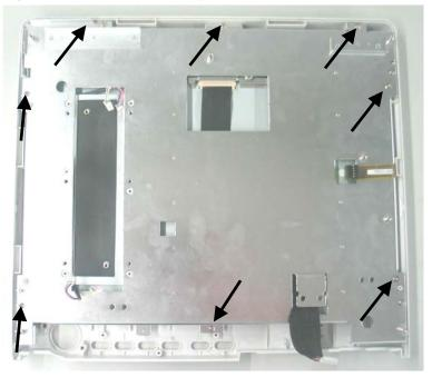
Unscrew the twelve M3×6 screws of T9 monitor and take the screen assembly out carefully. To prevent the screen from being contaminated by dust, do not touch the screen.
