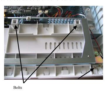
2. Pry the snaps out about 1mm away with a small flat-bladed screwdriver. Then insert the small flat-bladed screwdriver into the position marked in the picture and pry it out about 1mm so that the module rack becomes disengaged from the back cover.
