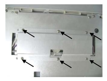
2. Unplug the cables respectively from the button board and the LCD to the inverter. Then, unscrew the two M3×6 screws to remove the inverter.
