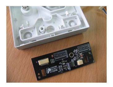
6. Unscrew the two screws on the front panel. Disconnect the tubing between the watertrap assembly and  $CO_2$  parameter board. Disconnect the cable between the watertrap and  $CO_2$  parameter board. Then take out the watertrap connector assembly.
