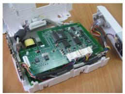
6. Take out the non-insulated power board and disconnect all the cables from it.
