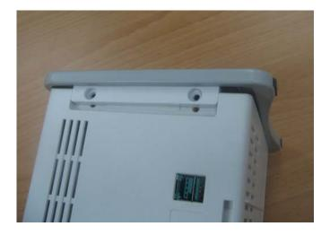
3. From the left side, remove the cable that connects the module rack interface board and the 8-slot module rack communication board. Then take off the SMR cover.
