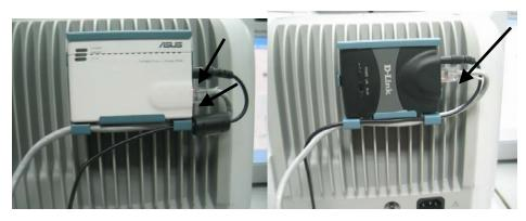
2. Press the leaf on the fix board with forceps; push the AP and installation board upwards. Then remove the AP and installation board.
