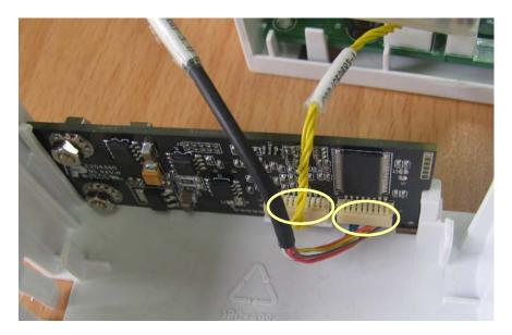
5. Disconnect the cables from the button board and unscrew the PT3×8 screw. Then release the two clips and take out the board. After that, disconnect the cable to the fan and remove the button board.
