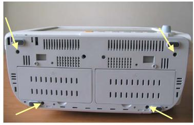
2. Pull out the base and then unplug the two cables marked in the picture, one connecting the Power Switch & LED board and the button board, and the other connecting the battery interface board and the power supply assembly.
