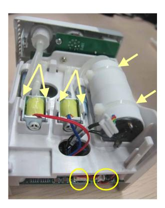
5. Unscrew the two  $M3\times8$  screws on the parameter board. Then pull off the parameter board rightward as shown below.
