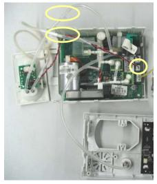
7. Disconnect the tubing between the  $CO_2$  parameter board and the front panel. Then release the four clips and remove the  $CO_2$  parameter board.
