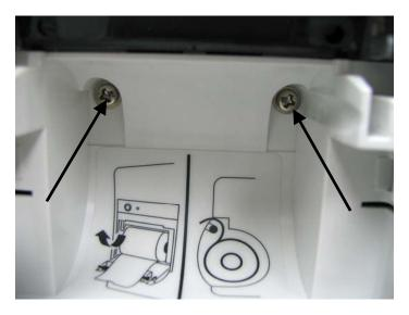
2. Pull the two clips in the directions as indicated and meanwhile pull out the recorder.
