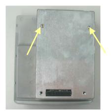
5. Unscrew the two M3×6 screws. pry out the board with a small flat-bladed screwdriver in the gap between the power supply board and the housing. Then turn the board over and unplug the cables from it.
