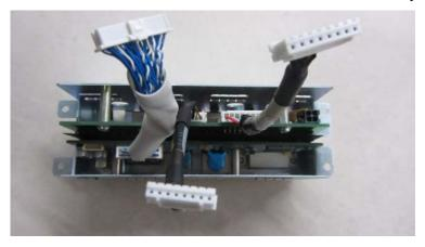
2. Unscrew the screws beside the DVI socket and micro-D socket. Then unscrew the two M3×6 screws in the holes. After that, pull out the DVI interface board.
