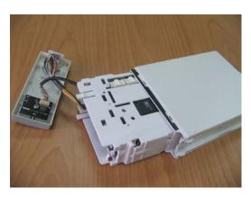
5. The side cover of the module without the housing is composed of two halves. Release the three snaps to separate the two halves.
