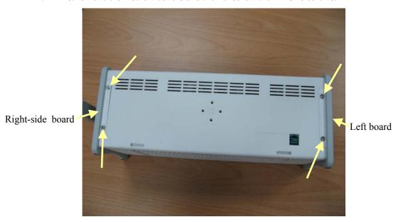
2. Pull off the left- and right-side boards. Be sure to place the rubber loop in position when reassembling the right board.
