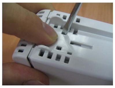
4. Press the two clips about 1mm and take off the housing.
