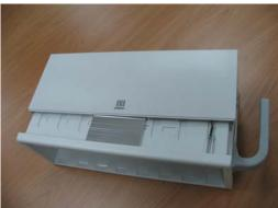
4. Unclench the two clips and take out the module rack interface board. Be sure not to damage the snap slot on the left side.
