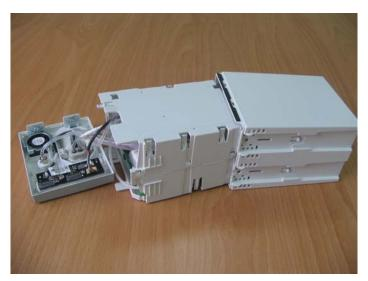
3. Hold the housing with both hands. Press the snap side with the thumb and move the other side with the index finger and the middle finger to separate the housing into two halves.
