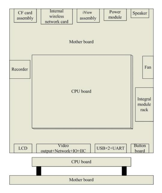
The CPU board is an essential CPU system containing the CPU, FLASH, memory, realtime clock, EEPROM, etc. It interfaces to the mother board only, which then provides interfaces to all other external devices.
