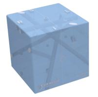
MultiPHAN features a set of rods for ease of registration, a ceramic central target, a ceramic offset target, and light field localization scribes.
