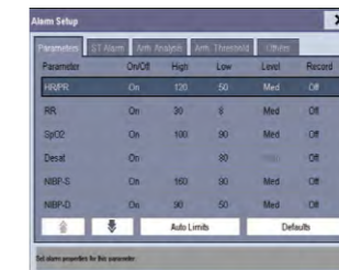
Mass alarm settings on one screen
